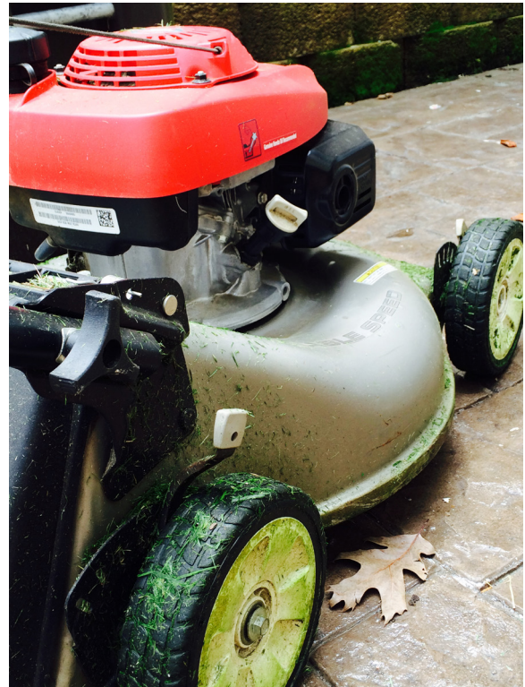
Image 2: Wheel adjustments on rotary mowers can raise or lower mowing height. Photo credit: J. Brosnan.
