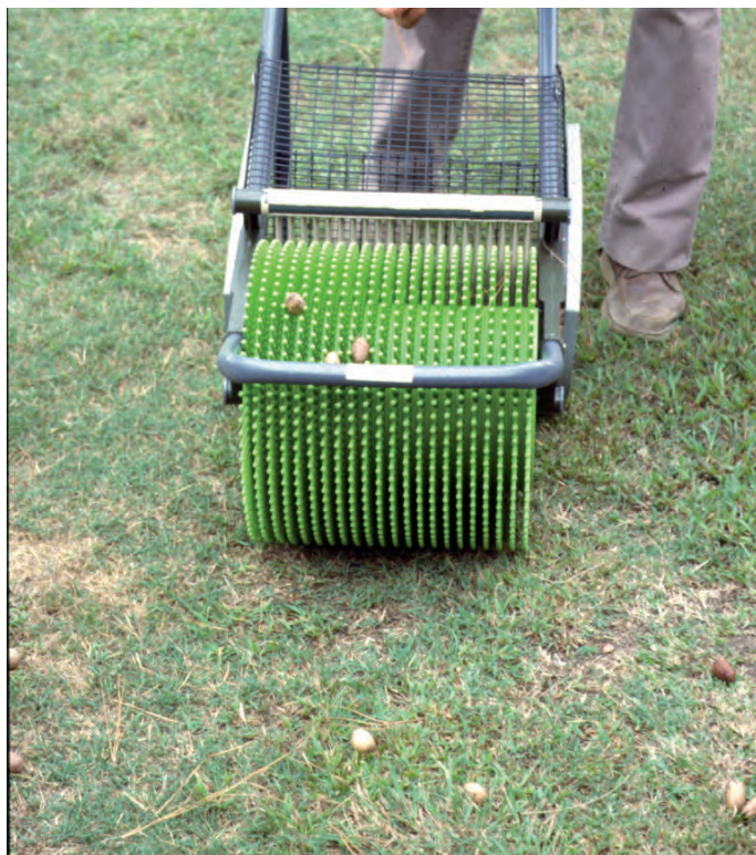
Figure 14. Example of a hand-pushed pecan harvester. Rubber bristles grab the pecans that are then brushed into the bin.
