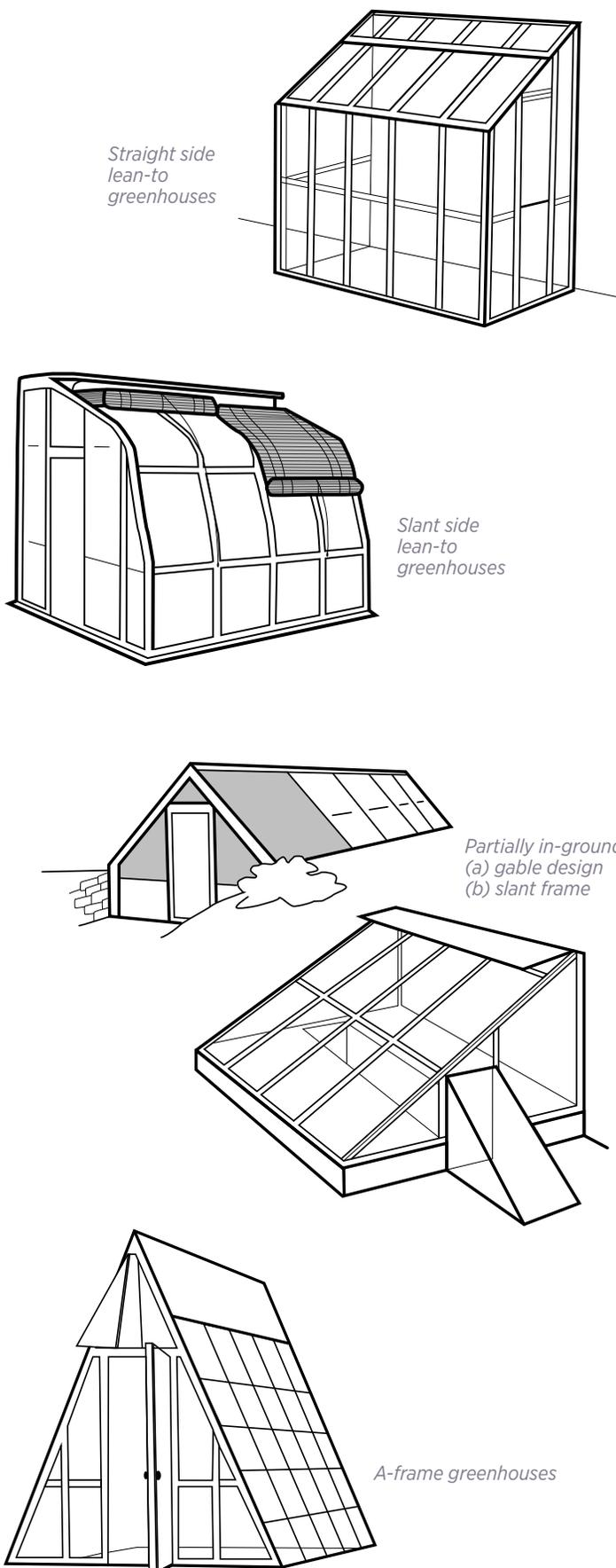
FIGURE 3. Examples of different designs for small greenhouses
