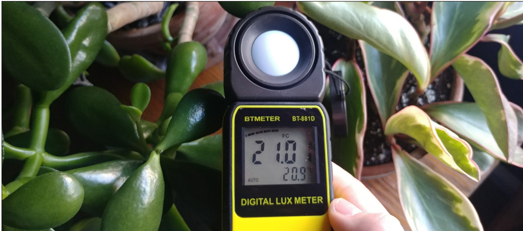
Figure 3. A simple, handheld light meter can be used to measure footcandles of light and determine suitability of a location for indoor plant growing. This reading of 21 footcandles taken in the winter in an east facing room is actually quite low and suggests the room may require some supplemental lighting.
